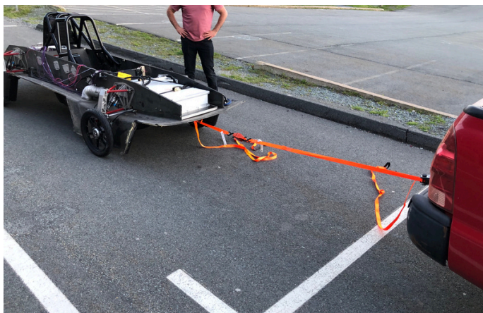
SEEN ABOVE: Dynamic testing of the parking break. Regulations require it to handle at least 10% of the car's total weight, or approx. 60lbs.
